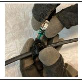
(a). Replace the old LED with new unit. Push the new LED into place.
