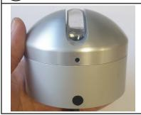
(a). Locate the two holes on each side of the MaxiEDGE.
