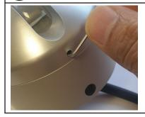
(a). Using a 1/16 Inch (1.5mm) hex key, loosen the grub screws. This will release the glare guard of the MaxiEDGE.
