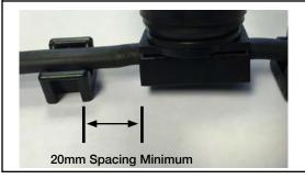
(a). Ensure that the Spacing between each Fixing Clip and MaxiLED Globe is 20mm Minimum
