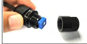
(a). Once the system is powered up and the DMX 512 data transmission is available the end of line units will need setting. Only perform this operation if the installation is flickering and not responding to the 512 DMX data transmission correctly. Remove the Black Cap.
